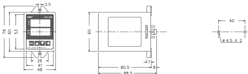
**Y type(Flush Mounting): Using US-08 Socket or P3G-08 Socket**
